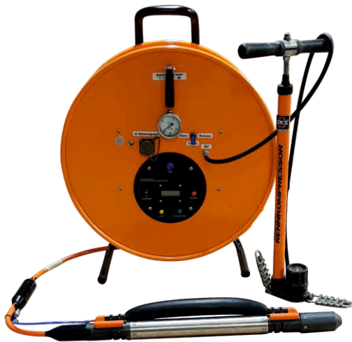
Borehole geophone BGK5 with cable drum and pneumatic clamping mechanism using an inflatable bladder.
